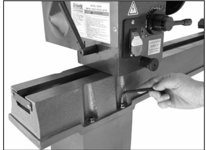
Figure 7. Securing lathe to stand legs.
